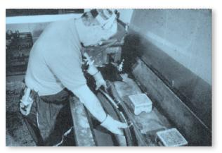
Hydrostatic hose testing.
