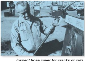
Inspect hose cover for cracks or cuts.
