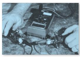
Hose assembly being tested with ohmmeter.
